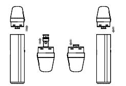
Remember to clean the condensation between the pod and the device.
